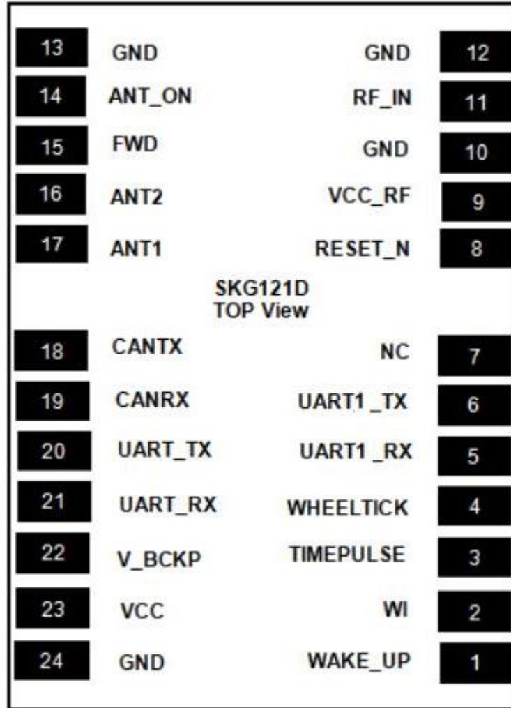
Figure 2: Pin Assignment
