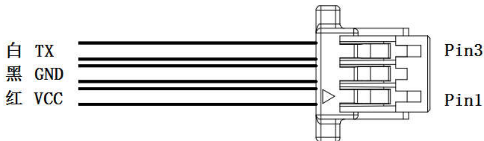
Figure 2: SKM81DC Pin Assignment
