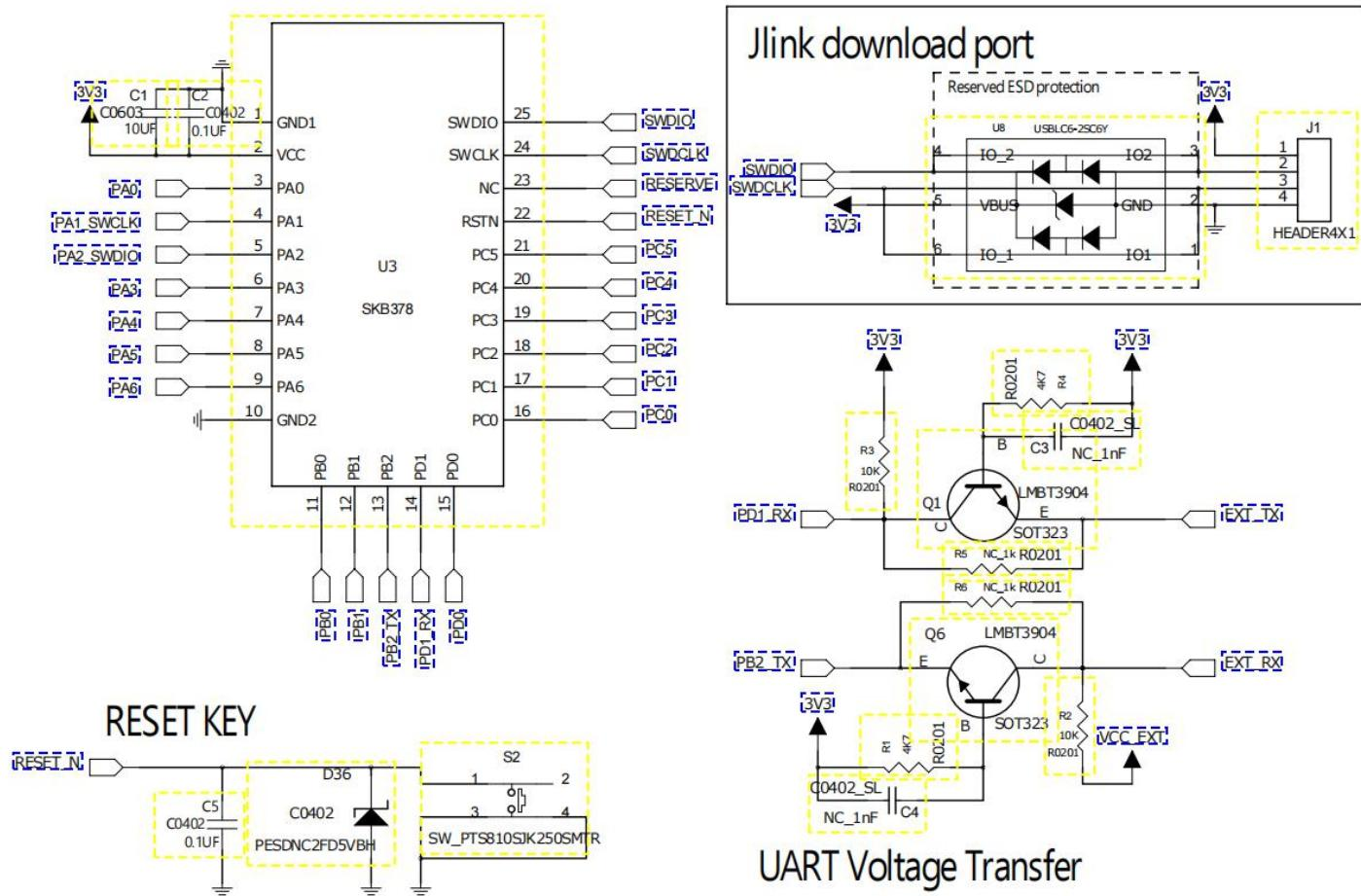
Figure 8 SKB378 Recommended Schematic
