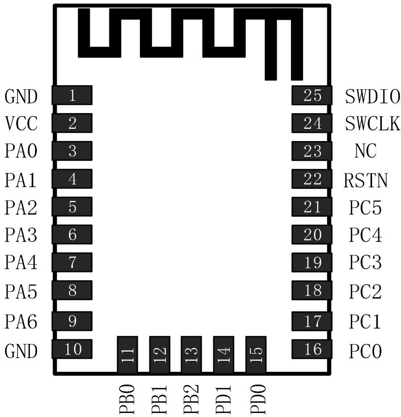
Figure 5.1: SKB378 Module Pinout
