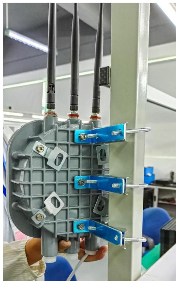
Figure3.1-R Insert the U-bolts to the L-shape steel
